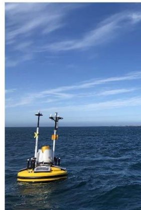
Accurate measurement of wind profile using SEAWATCH Wind LIDAR Buoy
