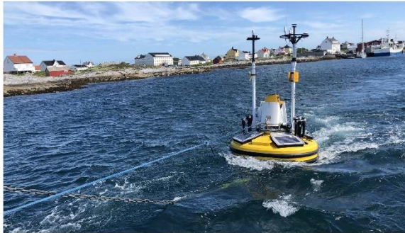
SEAWATCH Wind LIDAR Buoy towed in Frøya.
