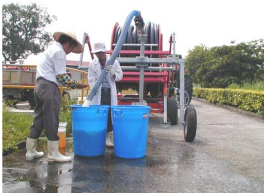
圖 3. 利用 100 L 之容器及馬錶測定在不同管線壓力下之噴灌流量。 Fig. 3. The flow rates of gun sprinkler under different terminal pressure were measured by 100 L of plastic tankers and timer.
